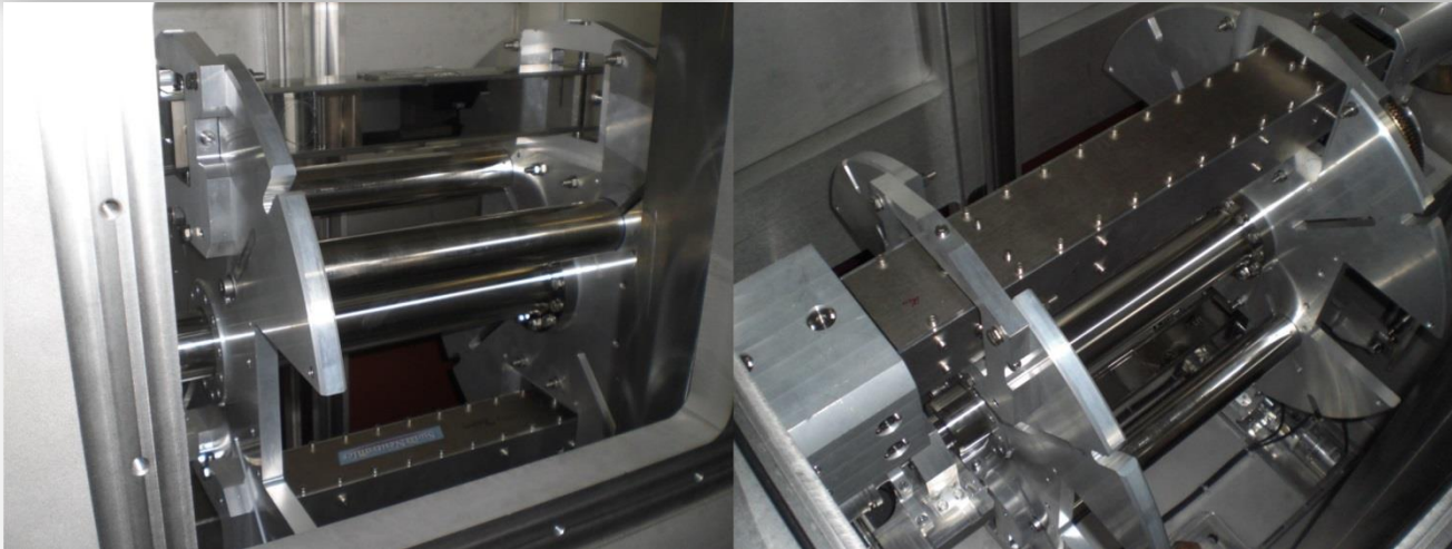
(left) Large cross-section radio-frequency spin flipper; (right) Polarizer chamber, chopper chamber and spin flipper; (bottom) Polarizer revolver with neutron guide and polarizer in beam;
