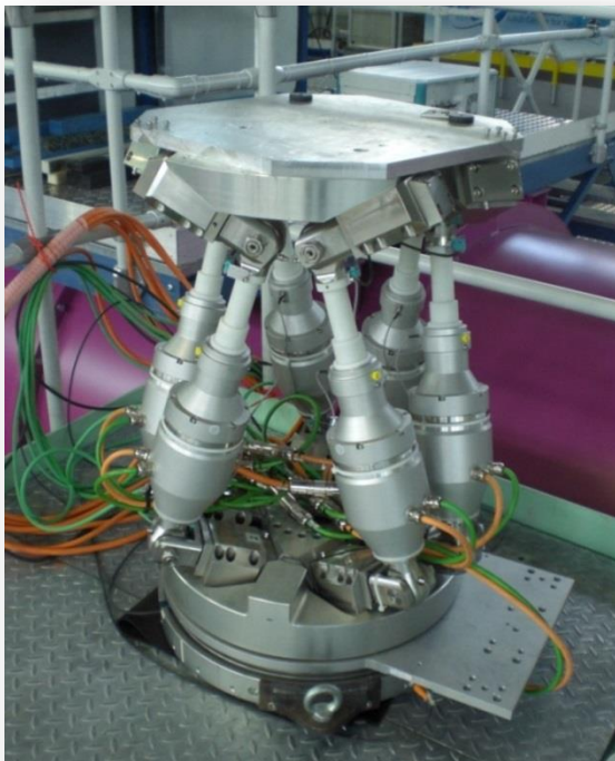
Hexapod (loading up to 550 kg)
