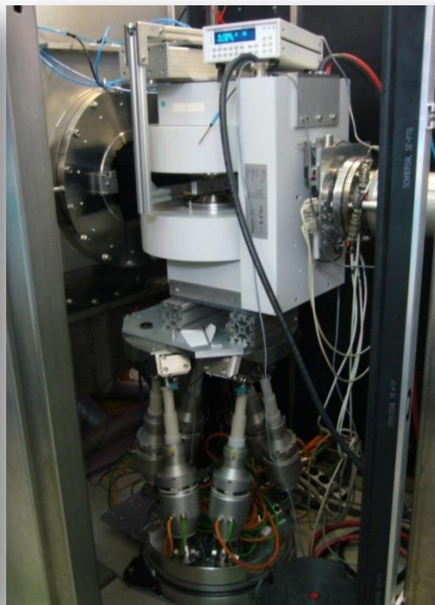
Electromagnet 2.2 T; has an option with cryofinger 10-320 K)
