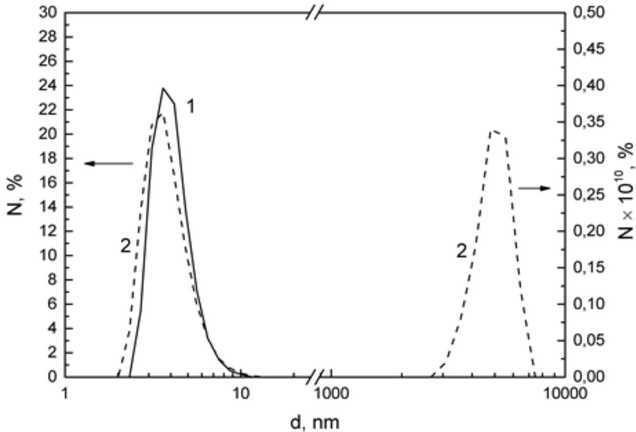
**Particles' fractions over size in Hydrosol (1) and Diamgel (2) prepared from this Hydrosol**
