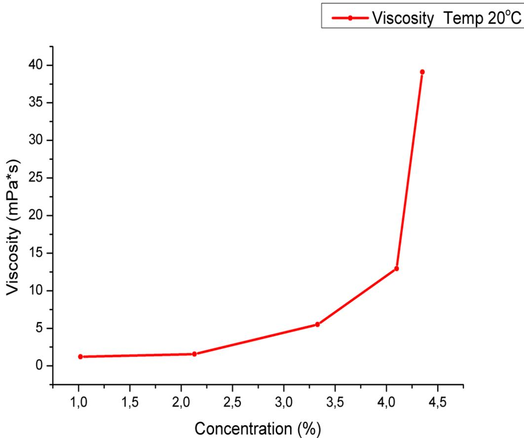
**High viscosity at low content of particles**
