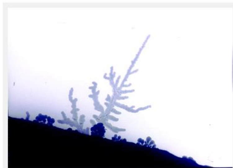
Actual lithium dendrites growing from an anode surface. Image from: R.R. Chianelli, J. Cryst. Growth, 1976, 34, 239-244.
