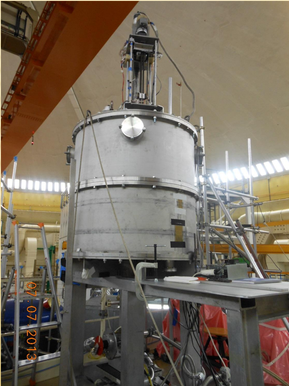
Vacuum chamber and filling system for new trap (ILL, Level D)
