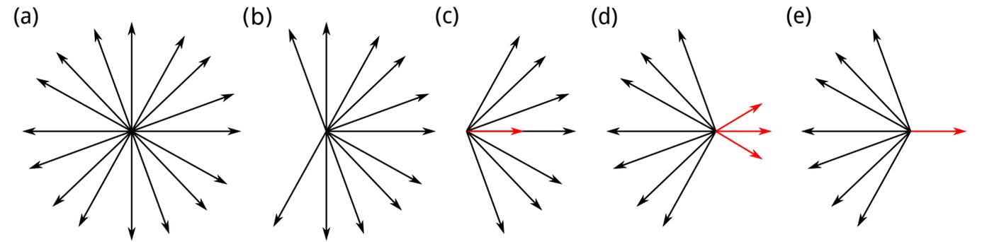
Figure 1 - Possible magnetic structures of magnetic amorphous alloys of RE-TM type: (a) — speromagnetic structure; (b) and (c) — asperomagnetic structure; (d) and (e) — sperimagnetic structure. Black and red arrows in (c), (d) and (e) subfigures represent different sublattices
