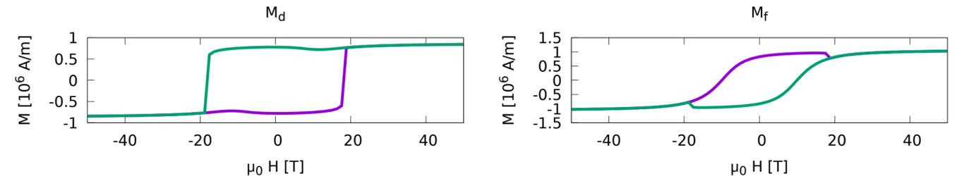
Figure 3 - Hysteresis loops of magnetizations for d- and f-sublattices for  $T=100$  K.
