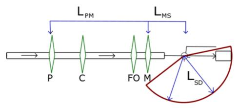
Before 2025: IN4 requires 1 transmission monitor and 1 square meter surface covered with helium-3 filled detector tubes.
