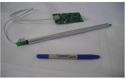
In 2019 the detector system for powder neutron diffractometer has been developed and manufactured to be installed on IR-8 reactor in Moscow in 2020. The detector system consist of 160 SiMP-based counters with sensitive area 5x50 mm<sup>2</sup>.
