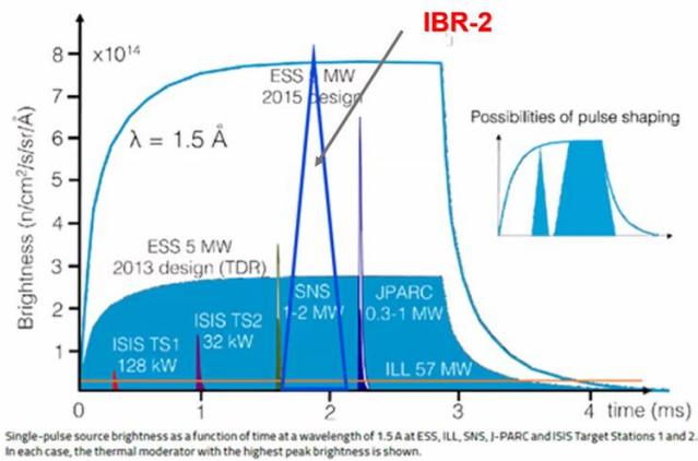
Single-pulse source brightness as a function of time at a wavelength of 1.5 Å at ESS, ILL, SNS, J-PARC and ISIS Target Stations 1 and 2. In each case, the thermal moderator with the highest peak brightness is shown.
