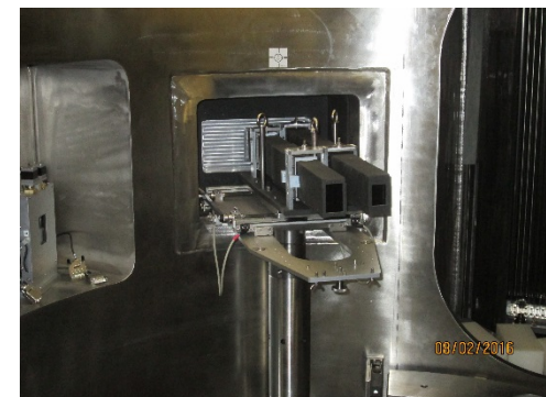
Exchange of the last section in the detector chamber
