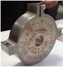
PMQ module for PRIOR : the magnetic field gradient – G=123 T/m at aperture of \varnothing 30 mm, nonlinearity of less than 0.7 %
