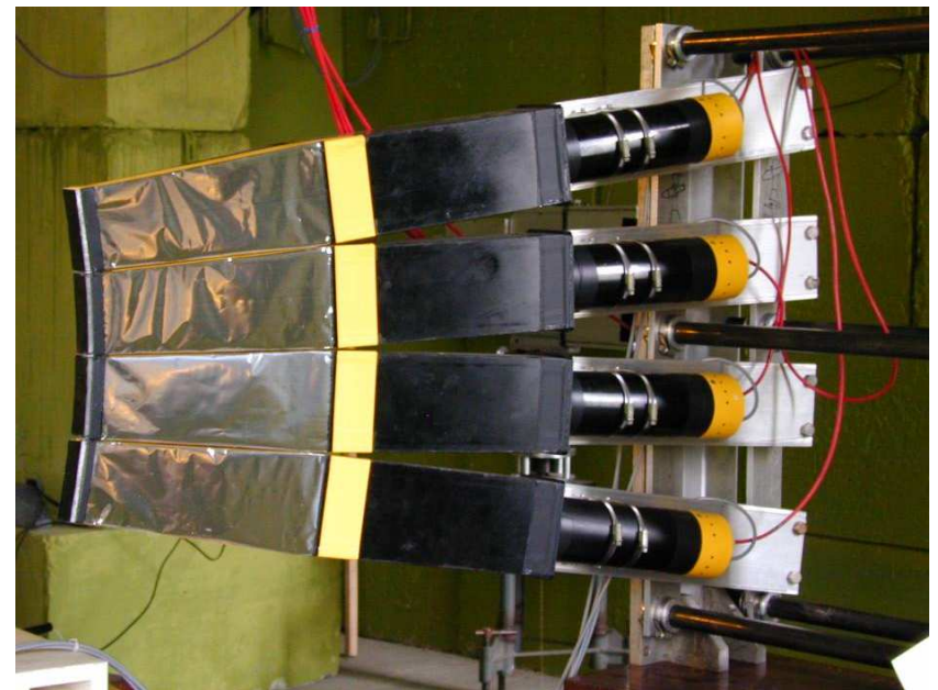
^6\text{Li} glass (old type) backscattering detector assembling on FSD.
