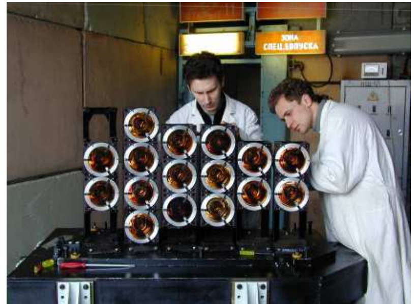
^6\text{Li} glass (old type) backscattering detector assembling on FSD.
