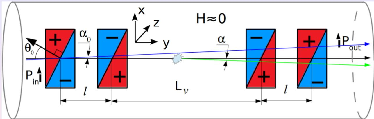
Single coil make a spin modulation in X direction  $\phi(x) = 2B\gamma_n \tan(\theta_0) \frac{x}{v}$
