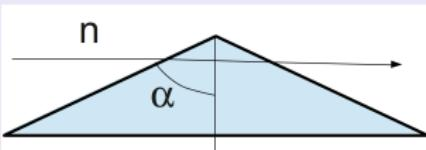
Value of phase shift due to refraction in prism
