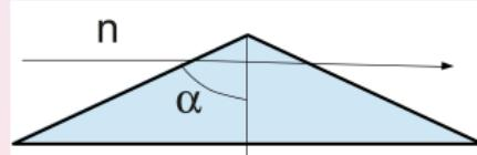
We use the quartz crystal prism with the vertex angle about  $156^\circ$  for neutron beam refraction.
