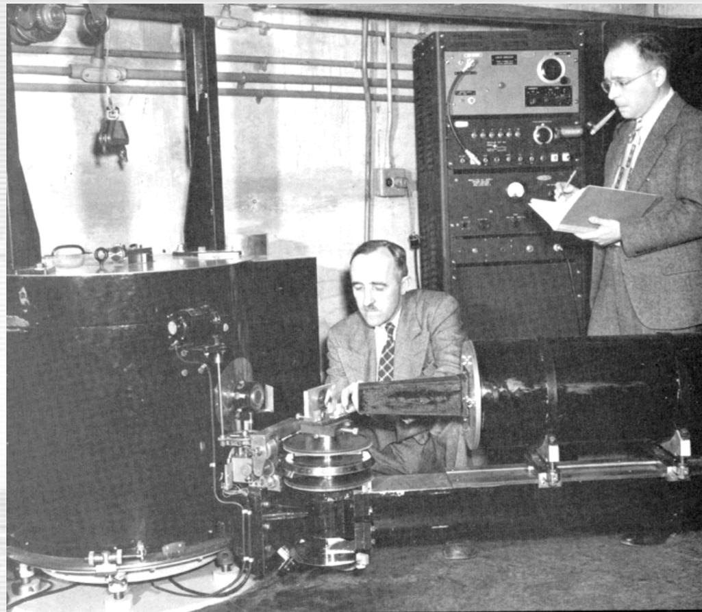
Ernest Wollan (left) and Clifford Shull (standing) working with their neutron diffraction unit at the Oak Ridge Graphite Reactor in 1950.
