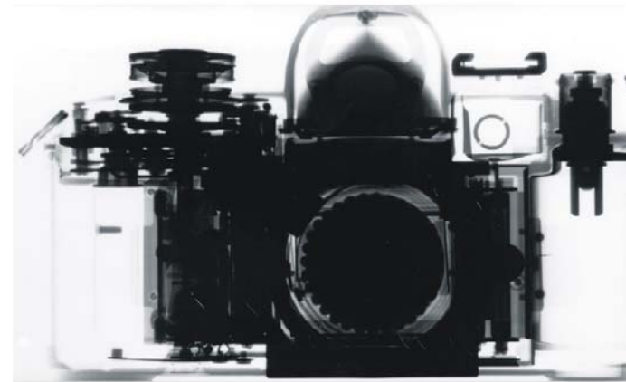
Fig. b: Radiographic image of a camera made X-rays
